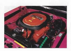
reasons) 290 hp tri-carb 340 cu in V-8, 4-speed Hurst-linkage manual (or optional Torqueflite automatic) transmission, Posi-Traction limited-slip differential, and a handling-tuned torsion-bar front, leaf-spring rear suspension. One of the first production cars with different-size tires front to rear, it wore E60-by-15 Goodyear Eagle STs in front and larger G60-by-15s in back to better manage the 340 V-8's ample off-the-line torque.
