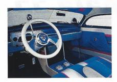
the sides "shaved," meaning all the trim and door handles are removed and the holes smoothly filled as if they were never there. The front bumper is '57 Chevy, the grille '54 Chevy with '53 teeth, the rear bumpers are four '55 Pontiac units, and the tail lamps are '71 Cadillac Eldorado. The interior boasts custom upholstery in white, blue, and fuchsia, high-tech liquid crystal gauges, a six-speaker Infinity sound system, and a tunnel-mounted 13-inch TV with VCR.
