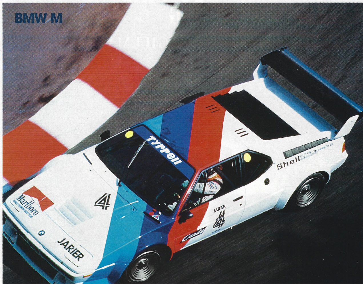
Racing versions of the M1 boasted an output of 470 hp and a top speed of 190 mph, well above the street version's 277 hp and 164 mph.
