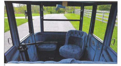
1-3. The 1919 Detroit Electric line included a Model 75B "doctor's coupe." Chassis equipment was in step with most other cars of the day, including leaf springs, beam axles, and friction shock absorbers. 4-6. Instrumentation was minimal, but seating was conducive to drivers who enjoyed company. Jill Eippert demonstrates the requisite tiller steering. Ease of operation made electrics popular with women. (Owners: Jill and Gary Eippert)
